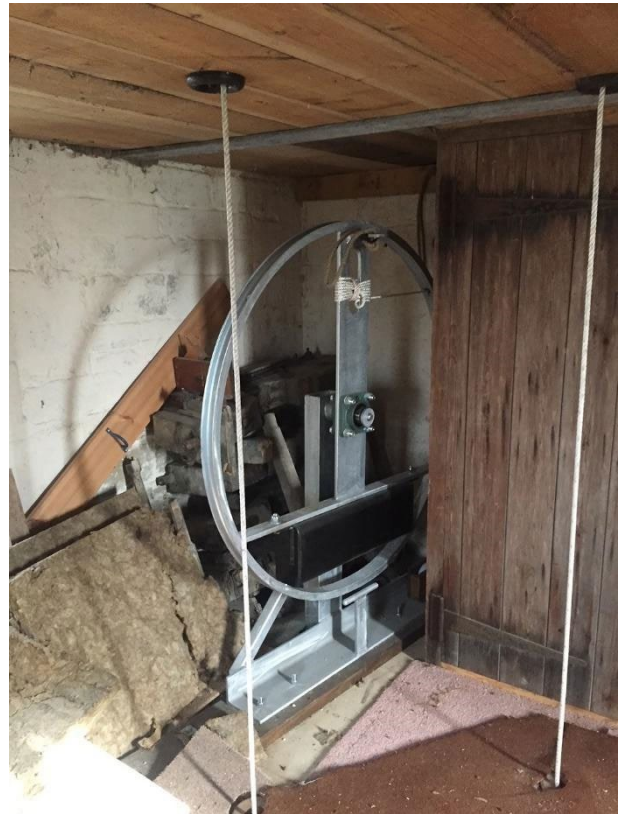
The training bell located unobtrusively in a corner of the clock room
